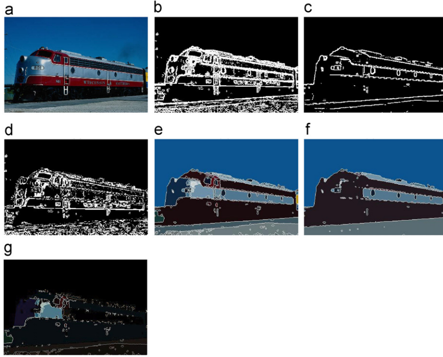
Fig. 6. An example of incremental image segmentation: (a) the original image; (b) and (c) are edge maps of (a) using the thresholds 80 and 150, respectively; (d) is the difference between (b) and (c); (e) and (f) are the segmented regions of (a) using the thresholds 80 and 150, respectively; and (g) is the difference between (e) and (f).
